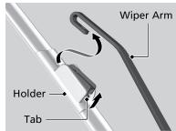
Pull the end of the wiper balde to the direction of the arrow in the image until it unfastens from the holder's end cap.
