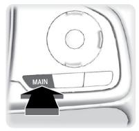
2. Accelerate to the desired speed (above 25 mph/40 km/h). Take your foot off the pedal and press the SET/- button to set the speed.
