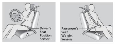
The driver's advanced airbag system includes a seat position sensor. Based on information from this sensor and the severity of the impact, the advanced airbag system determines the optimal deployment of the driver's airbag.
