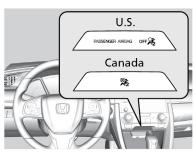
the indicator will come on and, in the event of a crash, the front passenger's airbag will not deploy.
