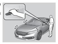
**To lock:** Press the door lock button on the front door
