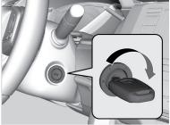
**Note:** The engine is harder to start in cold weather and in thinner air found at altitudes above 8,000 feet (2,400 m). When starting the engine in cold weather, turn off all electrical accessories such as the lights, climate control system, and rear defogger in order to reduce battery drain.
