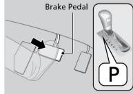
Press the ENGINE START/STOP button without depressing the accelerator pedal.
