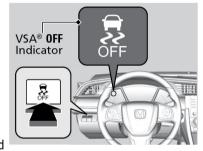
VSA® is turned on every time you start the engine, even if you previously turned it off. If you turn VSA® off, your vehicle has normal braking and cornering ability, but VSA® traction and stability enhancement become less effective.
