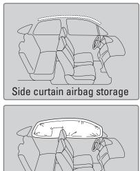
Deployed side curtain airbag
