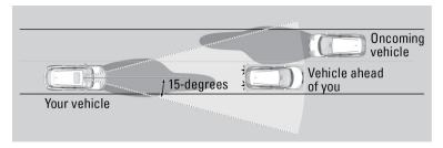
If a vehicle is detected ahead of you, the headlights stay in low beams. If the system does not detect any vehicles ahead of you, the headlights change to high beams.
