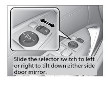
To enable reverse tilt, use the Vehicle Settings feature (See Customized Features)
