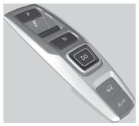
Drive /S Position(D)(D/S): Press the (D) button to put the vehicle in Drive. Release the electric parking brake to begin driving. Used for normal driving (D) or driving in Sport mode (S). Press D/S once for normal driving. Press
