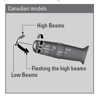
Push the lever forward to turn on the high beams.
