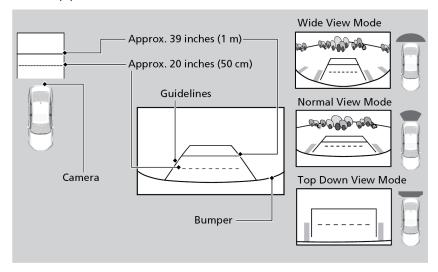
The rear camera view is restricted. You cannot see the corner ends of the bumper or what is underneath the bumper. Its unique lens also makes objects appear closer or farther than they actually are.
