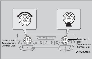
You can set the temperature synchronously for the driver's side and the passenger's side in synchronization mode.
