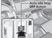
To turn the Auto Idle Stop system off, press this button. The Auto Idle Stop system stops.
