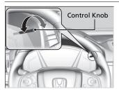
When the brightness of the meter will be reduced, you can use the brightness control knob to adjust instrument panel brightness. **Brighten:** Turn the knob to the right.
