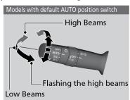
Push the lever forward to turn on the high beams.
