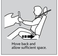
recommend that drivers allow at least 10 inches (25 cm) between the center of the steering wheel and the chest.
