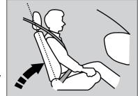
between the seat-back and your back. Doing so may interfere with proper seat belt or airbag operation.
