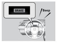
If a vehicle detected ahead of you slows down abruptly or if another vehicle cuts in front of you, the beeper sounds and a message appears on the driver information interface to alert you.
