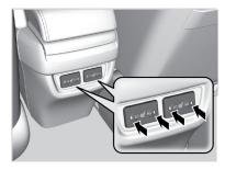
Do not use the seat heaters even in **LO** when the engine is off. Under such conditions, the battery may be weakened, making the engine difficult to start. In the **LO** setting, the heater runs continuously and does not automatically turn off.
