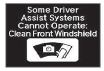
Anything covers the radar sensor cover or the area around the front sensor camera preventing detection of a vehicle in front. May appear when driving in bad weather (rain, snow, fog, etc.).
