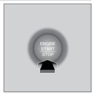
**Note:** The engine is harder to start in cold weather and in thinner air found at altitudes above 8,000 feet (2,400 m). When starting the engine in cold weather, turn off all electrical accessories such as the lights, climate control system, and rear defogger in order to reduce battery drain.
