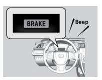
If a vehicle detected ahead of you slows down abruptly or if another vehicle cuts in front of you, the beeper sounds and a message appears on the driver information interface.
