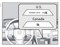
the passenger's front airbag will not deploy and the indicator will come on.
