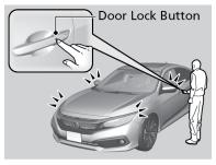
**Note:** System range is affected by radio signals from other devices (for example, cell phones or tablets) so for best results, carry the remote transmitter separately from these devices.
