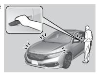
**To lock:** Press the door lock button on the front door. If the remote transmitter is inside the vehicle, the doors will not lock.
