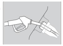
After filling, wait about five seconds before removing the filler nozzle.
