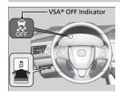
This button is on the driver side control panel. To partially disable VSA® functionality/ features, press and hold it until you hear a beep.
