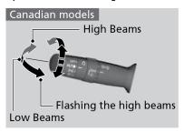
Push the lever forward to turn on the high beams.
