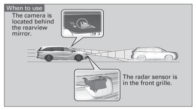
When a potential collision to an oncoming detected vehicle is determined, the system alerts you with rapid vibration on the steering wheel, in addition to visual and audible alerts. Take appropriate action to prevent a collision (apply the brakes, operate the steering wheel, etc.).
