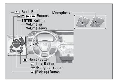
Pick-up button: Press to go directly to the phone screen of the driver
