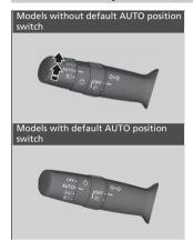
Automatic lighting control can be used when the power mode is in ON.
