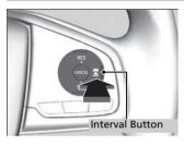
Press the 🖹 (Interval) button to change the ACC with Low Speed Follow following-interval.
