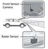
The radar sensor is inside the front grille.
