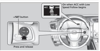
When driving at about 25 mph (40 km/h) or above: Take your foot off the pedal and press the -/SET button when you reach the desired speed. The moment you release the button, the set speed is fixed, and ACC with Low Speed Follow begins.
