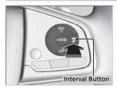
Press the 🖹 (Interval) button to change the ACC with Low Speed Follow followinginterval. Each time you press the button, the following-
