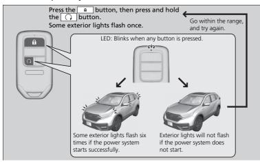
The power system is on for up to 10 minutes without you starting the vehicle. To extend the time for another 10 minutes during the first 10 minutes, press the a button, then press and hold the \(\bigcap\) button.
