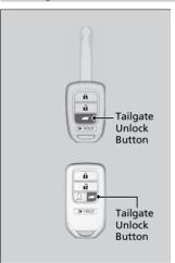
Press the tailgate unlock button to unlock the tailgate.
