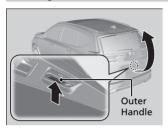
When all the doors are unlocked or press the tailgate unlock button on the remote transmitter, the tailgate is unlocked. Press the outer handle and lift open the tailgate.
