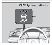
When VSA® activates, you may notice that the engine does not respond to the accelerator. You may also notice some noise from the hydraulic brake system. You will also see the indicator blink.
