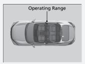
The engine may also run if the smart entry remote is close to the door or window, even if it is outside the vehicle.
