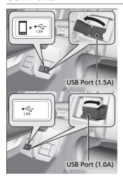
Install the device USB connector or the USB flash drive to the USB port.
