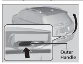
If you press the outer handle of the tailgate for no longer than one second, the tailgate opens automatically.
