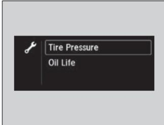
Shows the current condition of the tire pressure and the remaining oil life.
