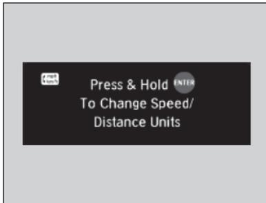
Enables you to set the speedometer and the displayed measurements to read in either mph or km/h.
