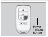
Press the power tailgate button for more than one second to operate when the power mode is in VEHICLE OFF (LOCK).
