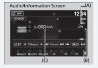
(A): Shows how much time the replayed segment is behind the real-time broadcast(B): Replayed segment(C): Length stored in memory
