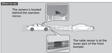
The system starts monitoring the roadway ahead when your vehicle speed is about 3 mph (5 km/h) or above and will search for a vehicle in front of you.
