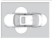
When you carry the keyless remote, you can lock/unlock the doors and fuel fill door, and open the trunk.
