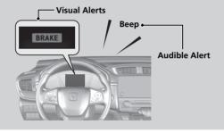
You can change the distance (**Long/Normal/Short**) between vehicles at which the system's earliest collision alert will come on through the driver information interface\* or the audio/information screen\* setting options.
