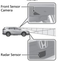
The radar sensor is inside the front arille.
