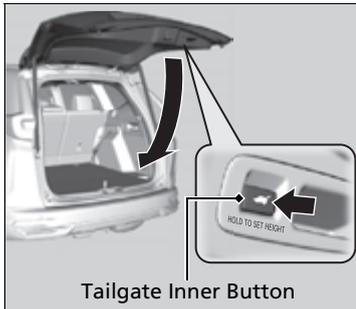
Press the tailgate inner button on the tailgate to close the power tailgate.
