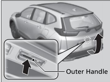
When all the doors are unlocked or you press the tailgate unlock button on the remote transmitter, the tailgate is unlocked. Press the outer handle and lift open the tailgate.
