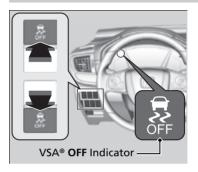
This button is on the driver side control panel. To partially disable VSA® functionality/ features, press and hold it until you hear a beep.
