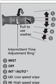
The windshield wipers and washers can be used when the power mode is in ON.
