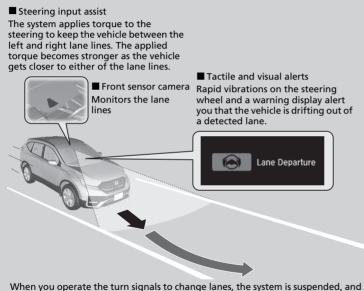
When you operate the turn signals to change lanes, the system is suspended, and resumes after the signals are off.
